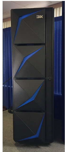
Figure 4.2 A single-frame IBM z15 mainframe. Larger-capacity models can have up to four total frames. Source: Agiorgio/Wikimedia Commons/CC BY-SA 4.0.
