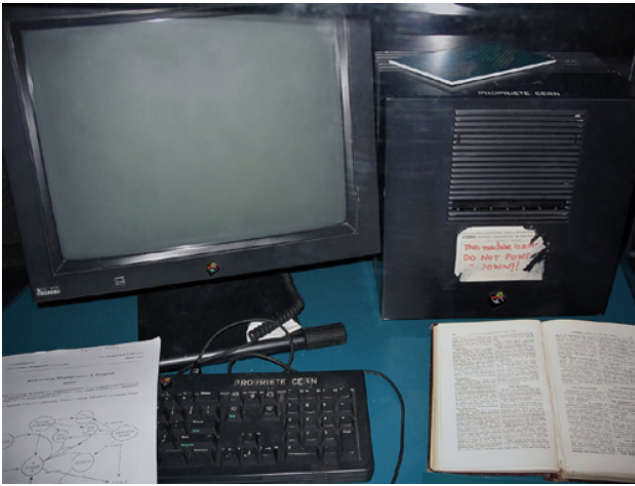
Figure 4.4 The world's first Web server, a NeXT Computer workstation with Ethernet, 1990. The case label reads: 'This machine is a server. DO NOT POWER IT DOWN!!'. Source: Coolcaesar Wikimedia Commons/CC BY-SA 3.0.
